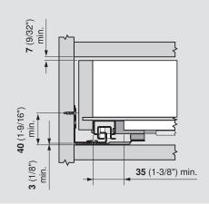
NOTE: TANDEM runners will sit 3 (1/8") higher when using the lateral stabilizer in bottom mount applications and may have to be raised for some bottom mount drawer applications using SERVO-DRIVE
