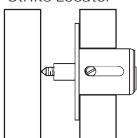
Use strike locator to correctly mark location to install strike.
