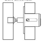
Use optional bolt extender for excessive gaps in bypassing doors.
