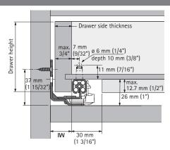
▶ Installation recommended with one #6 - #8 flat head or Ø 6.3 x 14 mm Euro screw per side
