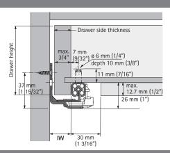
▶ Installation recommended with two #6 - #8 flat head or Ø 6.3 x 14 mm Euro screws per side
